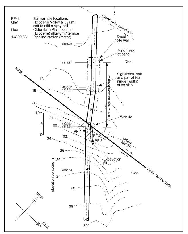
Figure 4. Pipeline and Fault Location After Earthquake.
