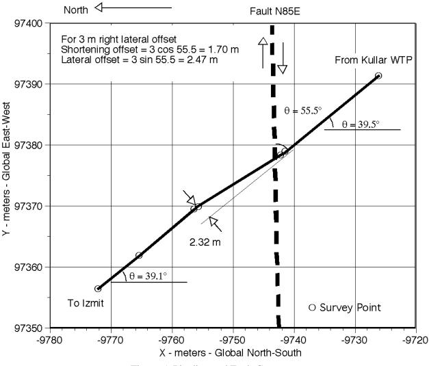
Figure 5. Pipeline and Fault Geometry
