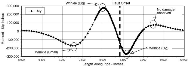
Figure 6. Variation of Bending Moment along the Pipeline Near the Fault, Model 4
