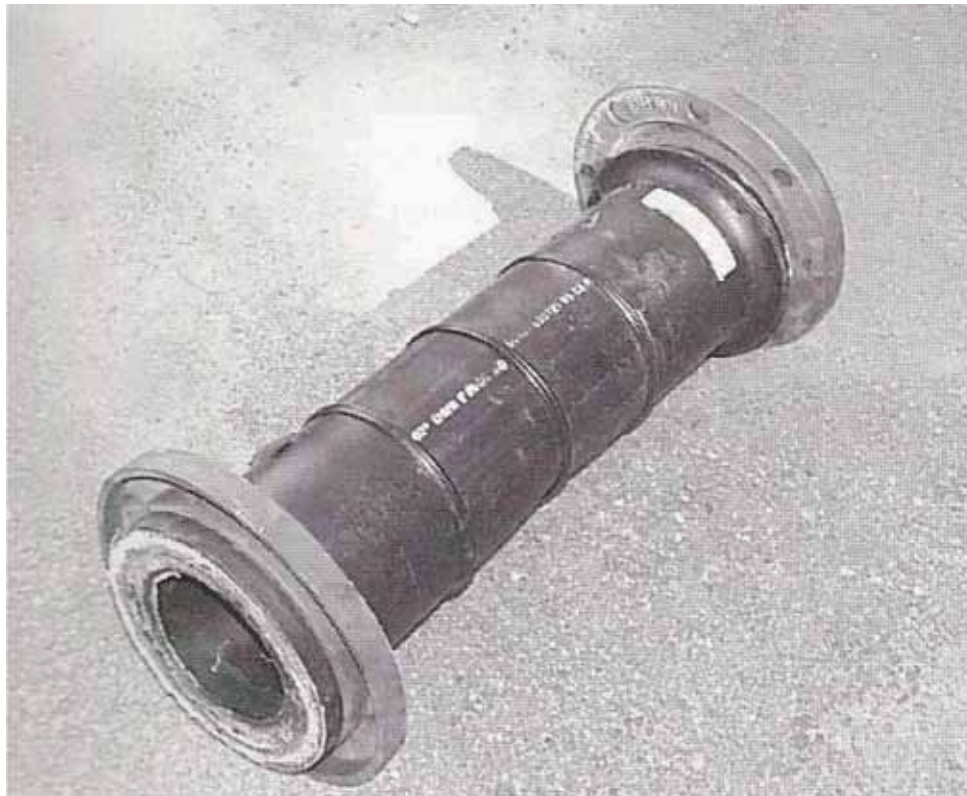
Figure 10-8. PE Pipe with Three Fusion Butt Welded Joints
