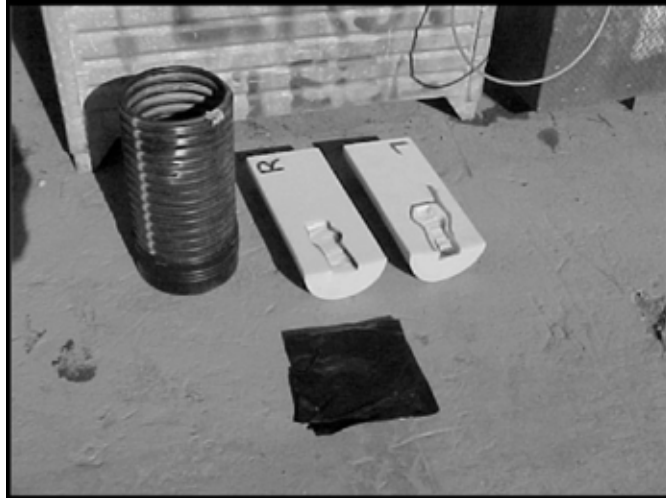
Figure 11-10. Photo of service boot components: HDPE drain pipe and end cap (upper left), two foam inserts (upper right), and visqueen sheeting (foreground)
